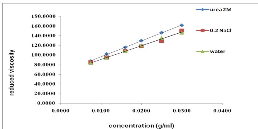
Figure 5: Viscosity of dextran in different solvents.
