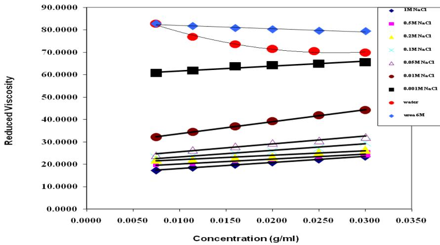
Figure 2: Viscosity of *A. senegal* gum in different solvents.
