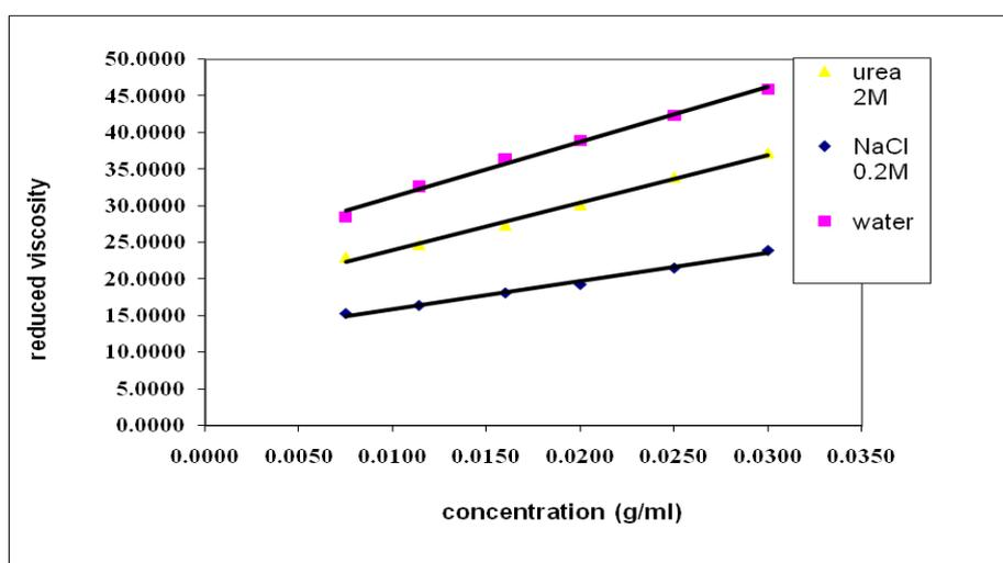
Figure 6: Viscosity of sodium caseinate in different solvents.
