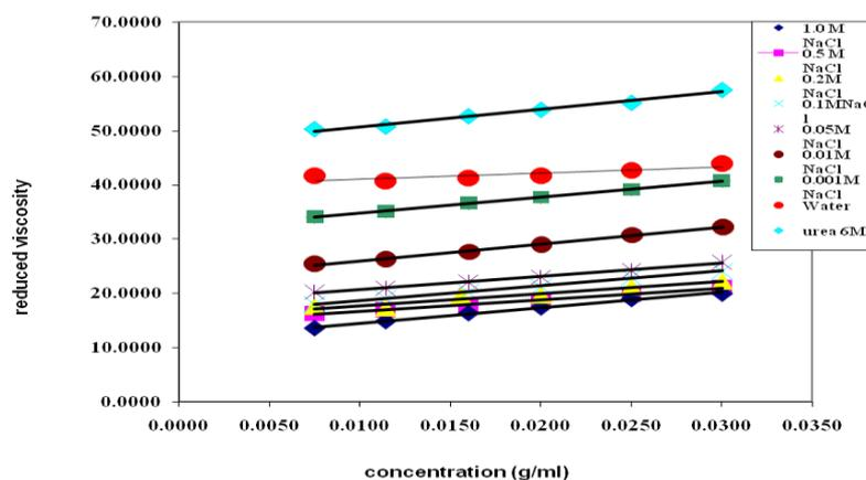
**Figure 1: Viscosity of *A. seyal* gum in different solvents.**
